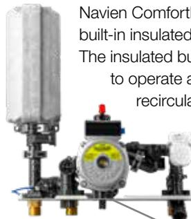
Navien ComfortFlow® is the first to incorporate a built-in insulated buffer tank and recirculation pump. The insulated buffer tank enables the NPE-A2 to operate at minimal flow rates. The built-in recirculation pump allows the NPE-A2 to recirculate water either through an external recirc line or through existing supply lines while using NaviCirc™, without the need for external pumps or controls.
