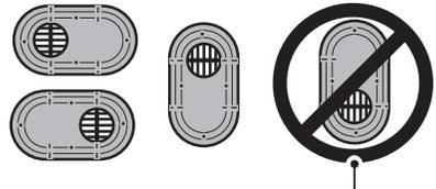
NEVER install in this orientation with the exhaust located nearest to the ground.
