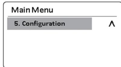
2. Press the Up button (▲) or the Down button (▼) to switch between information items. Press the OK Button (OK) to select an item to view the information.
