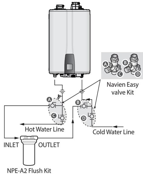
To flush the Heat Exchanger: NPE-S2 Model
