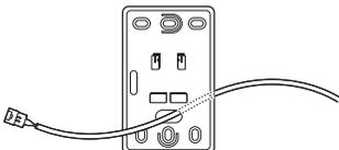
3. Connect the end of the extension cable to the cable connected to the remote controller.
