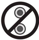
Do not vertically stack concentric terminations on sidewalls. The circulation of exhaust gases will cause improper operation of the water heater.
