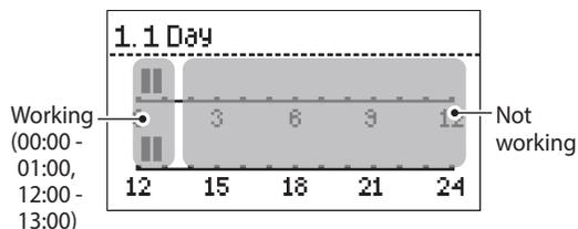
Press the Up button (▲) or the Down button (▼) to choose the scheduled time. You can choose the time in 30 minutes intervals. To finalize the weekly schedule settings, press and hold the OK button (OK) for more than 2 seconds.
